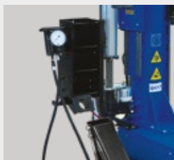
Foot pedal operated inflation control gauge and wheel balancer valve.
