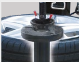
Clamping mechanism with two heights for standard rims or with reverse rims.
