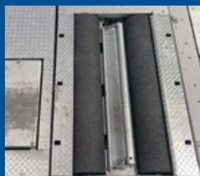
Rollers with crystalline silicon resin coating.
