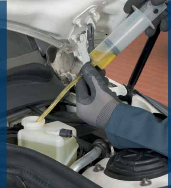
Checking the brake-fluid level at the expansion tank
