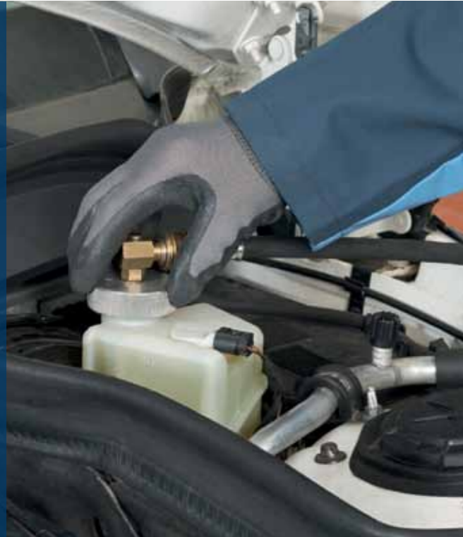
Connecting the overpressure equipment
