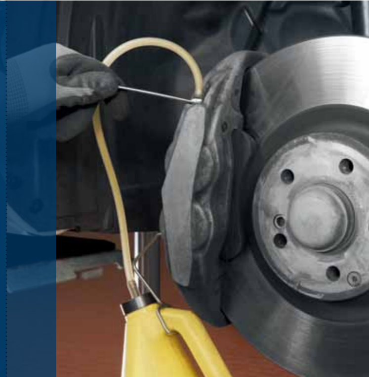
New brake fluid flows in – free of bubbles and yellow
