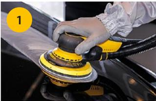
Remove defects: use Microstar® grit P1200 or P1500 + 5 mm interface pad. Sand with medium speed, 6,000–7,000 rpm.
