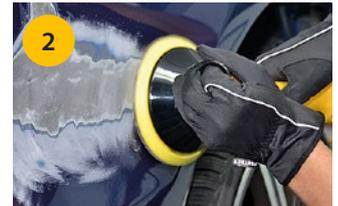
Remove paint on repair area, use net disc grit P80 or P120.
