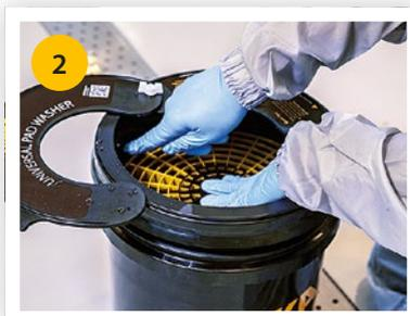
➤ Press down the washing grid and fill the bucket with water until it is slightly above the washing grid.
