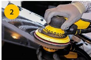
Reduce scratches: use Abralon® grit 3000 damp sanding. Sand with low speed, 6,000 rpm.
