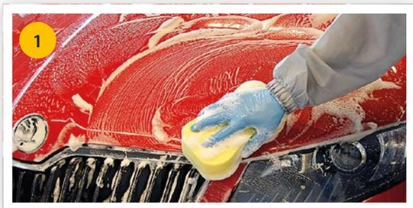
» Wash your car carefully. A dirty lacquer surface causes scratches when polishing and affects the final result.
