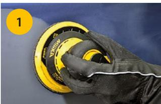
1 Preparation of adjacent panels and panel blend. Use Abralon® grit 1000 disc damp or Polarstar®/Microstar® disc with interface pad dry.
