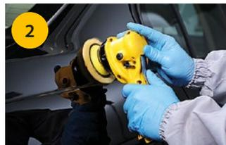
Gentle press on the machine at moderate speed, wipe clean and check the surface. Repeat the compounding process if needed.
