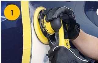
1 Sand repair area expanding feather edge into original paint work. Use disc grit P320 with a soft interface pad.
