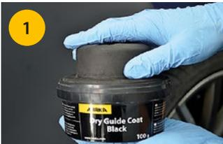
1 Apply Mirka Dry Guide Coat to highlight scratches from previous sanding step.
