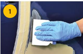
Mix and apply filler to damaged area, avoiding surrounding paintwork.
