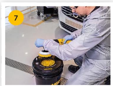
➤ For additional drying place the center grid in the lid. Recommended speed: 1,200 – 1,500 rpm.
