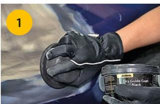
Apply Mirka Dry Guide Coat on filler area.
