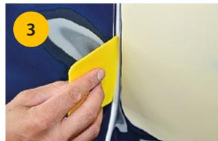
3 Adjust the foam tape for best masking result.
