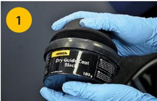
1 Apply Mirka Dry Guide coat on the primer filler area.
