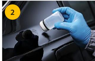
Always use water when sanding, apply water to both abrasive and on defect area. Use Mirka damper for best result.
