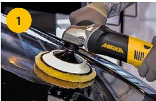
Use Polarshine® 10 and Mirka® Lambswool Pro pad. Polishing speed max. 1,500 rpm.
