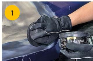
Apply Mirka Dry Guide Coat to highlight imperfections on the surface.
