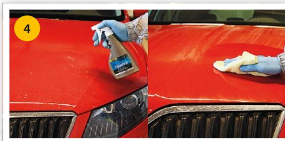
» Spray a small amount of wax on the surfaces. Spread out and dry with a microfibre cloth.
