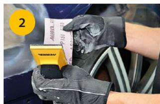
Fine sanding of body filler and feather out. Use net strip grit P180–P240 with sanding block or Mirka® DEOS 383 machine. >>> Check repair area, if required fill pinholes with a fine polyester filler.
