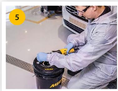
➤ Press down the polisher against the grid and run the polisher at approximately 800 – 1,200 rpm.
