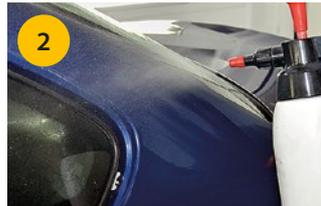
Preparation is the key. Degrease the whole working area.
