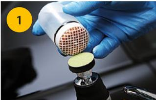
For removing of defect use Polarstar® SR and Mirka® AOS 130NV or AOS-B 130NV machine.
