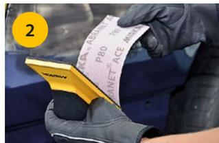
Shape and level body filler. Use net strip grit P80 or P120 with sanding block or Mirka® DEOS 383 machine.
