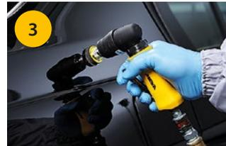
Light press with machine and sand for 2-3 seconds.
