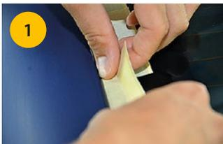
1 If needed, use Perforated Lifting Tape for rubber trims.
