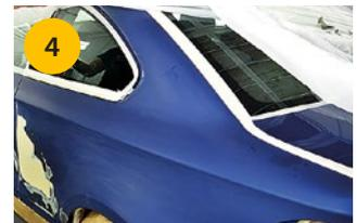
4 Protect the rest of the vehicle with Masking Film or Premium Masking Film.
