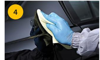
Wipe clean and check the surface. Repeat step 3 if needed. Use Mirka soft microfiber cloth.
