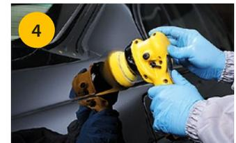
Gentle press on the machine and use at moderate speed, wipe clean and check the surface. Repeat the polishing process if needed. Use Mirka soft microfiber cloth for final cleaning.
