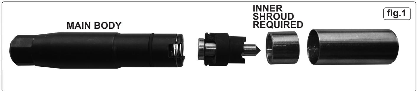
**NOTE:** Apply tape to outer shroud.
