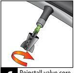
Reinstall valve core.
