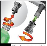
Slowly remove valve core with tool in cap.
