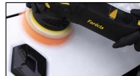
Spread the product on the surface, then polish flat at 3000opm ( setting 3 on the G Plus Dual Action Polishing Machine GPT203 ).
